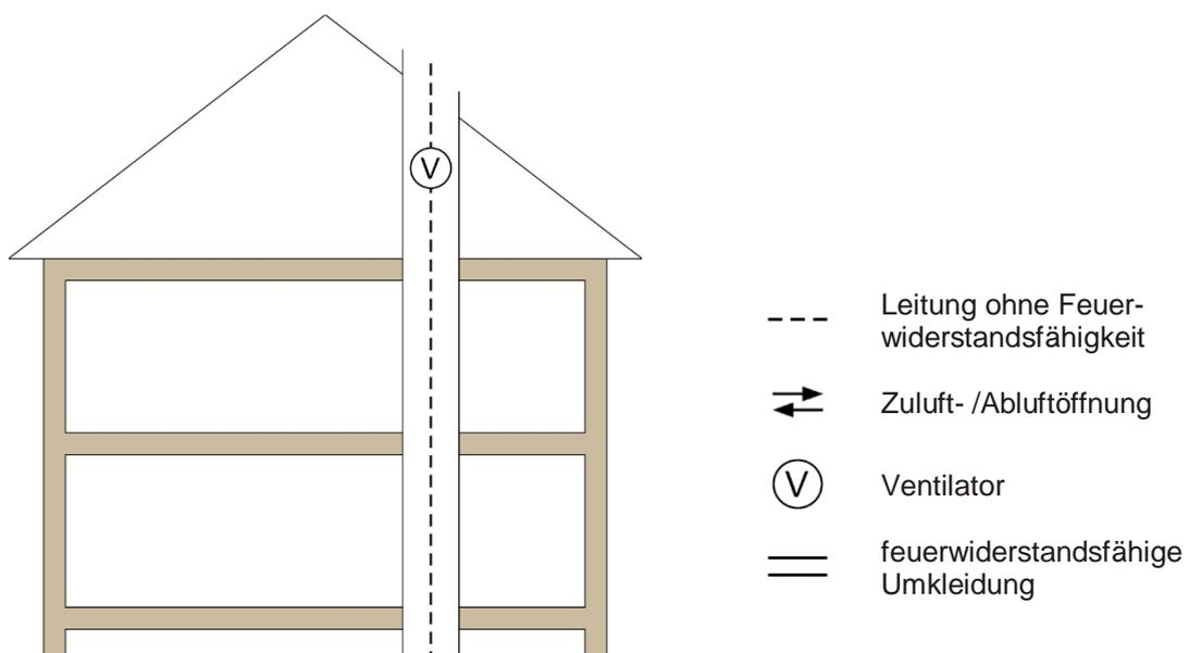
**Bild 3.2: notwendiger Flur belüftet**
